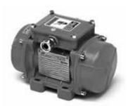
These electric vibrators are designed and built to withstand the rigors of the industrial environment and operate in a continuous duty cycle. This series is so tough we guarantee them for 3 years even when operated at 100% amplitude setting, in a 24/7 operating environment. Each vibrator is manufactured using the latest automated techniques, insuring exact bearing and seal fits. Add vacuum impregnated windings and you have a high performance vibrator second to none.
