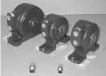
Gruber Pneumatic Ball Type Vibrators are used to vibrate excess air out of the marble matrix after pouring. Gruber Vibrators provide high-frequency vibration at an economical price. The only moving part is a high-grade chrome steel ball. Lubrication, while not required, extends the life of the units. Other uses for these vibrators are for small hoppers, parts feeders, chutes and match plates. Air consumption for these units is moderate.
