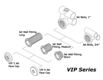
VIP 3 Jets are assemblies of three individual components - a Jet Body, a Wall Fitting, and a VIP 3 (or VIP 4) style Facecap.
