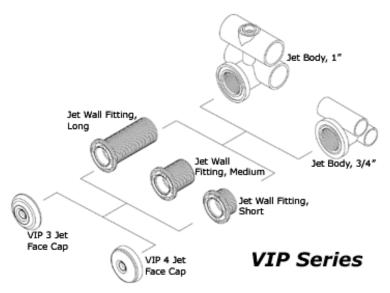
The illustration (at left) shows the three components - and shows a choice of both Jet Bodies, and Wall Fittings. Which one of each is right for you depends on the pump and water hose used in your system, and thickness of the bath tub you are adding the whirlpool kit to. Note that VIP 3 and VIP 4 facecaps are interchangeable on a VIP jet system.
