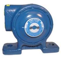
**Model CV-25** - extra heavy-duty construction for operation in adverse conditions or water, heat, cold and grit. Vibration is controlled from a few cycles per minute to full speed by installation of a needle valve or pressure regulator. These vibrators assure satisfactory and efficient vibration for the toughest jobs. Order No. - 02012
